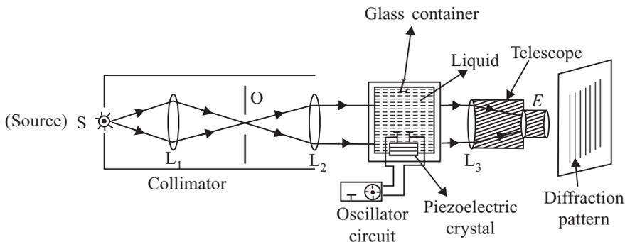
**Fig. 1.6** Schematic diagram of acoustic grating
