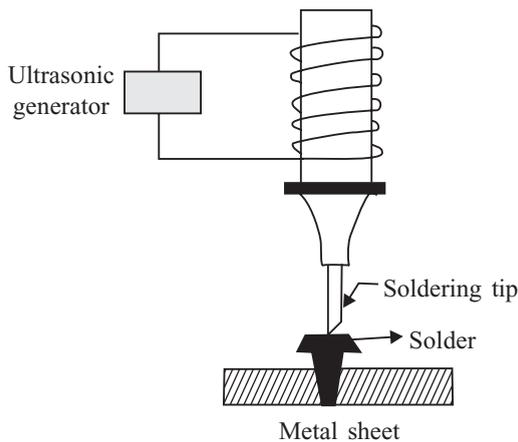
**Fig. 1.9** Ultrasonic soldering system
