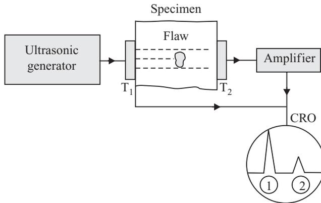
**Fig. 1.12** Schematic diagram of the transmission technique
