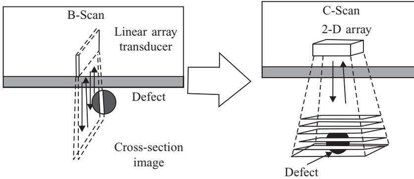
**Fig. 1.17** Difference between a B-scan and a C-scan
