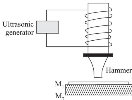
**Fig. 1.8** Ultrasonic welding system
