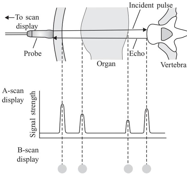
**Fig. 1.15** Schematic representation of A-scan and B-scan displays
