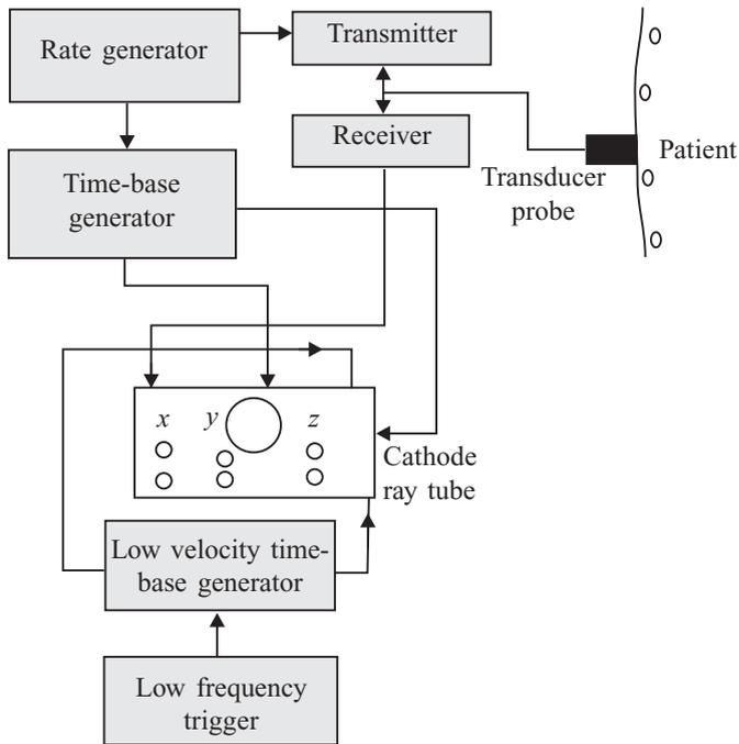
**Fig. 1.13** Block diagram of an echocardiograph unit
