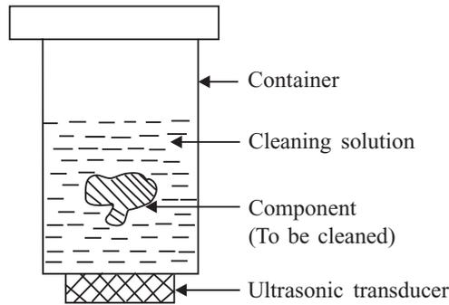
**Fig. 1.10** Ultrasonic cleaning system
