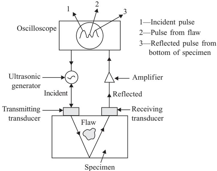
**Fig. 1.11** Ultrasonic flaw detection system
