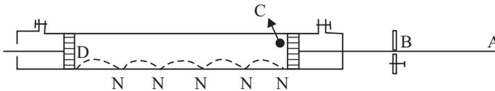
**Fig. 1.5** Kundt's tube set-up for detection of ultrasonic waves
