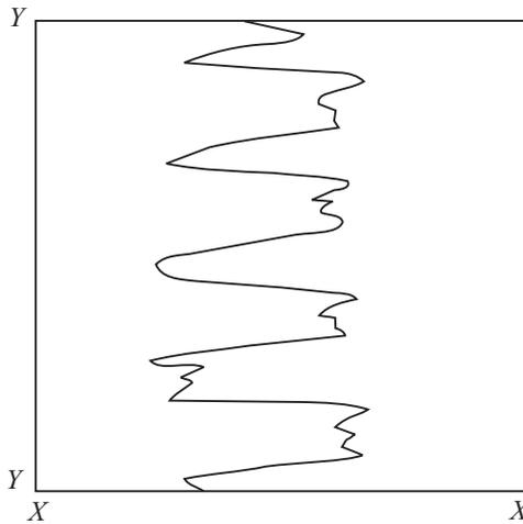
**Fig. 1.14** Typical zigzag movement of the CRT spot
