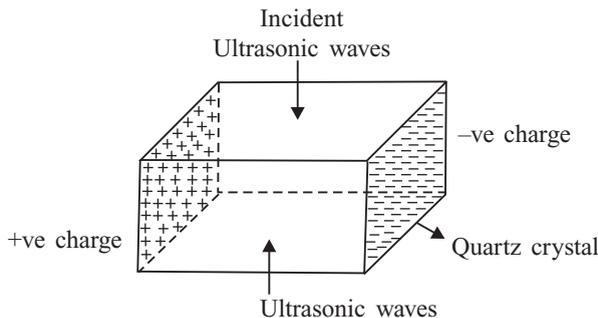
**Fig. 1.4** Schematic representation of piezoelectric detector
