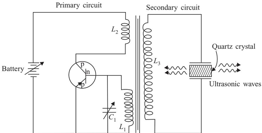
**Fig. 1.3** Piezoelectric oscillator circuit
