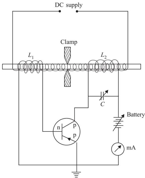
**Fig. 1.2** Circuit diagram of magnetostriction method
