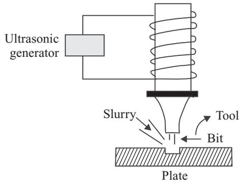
**Fig. 1.7** Ultrasonic drilling system
